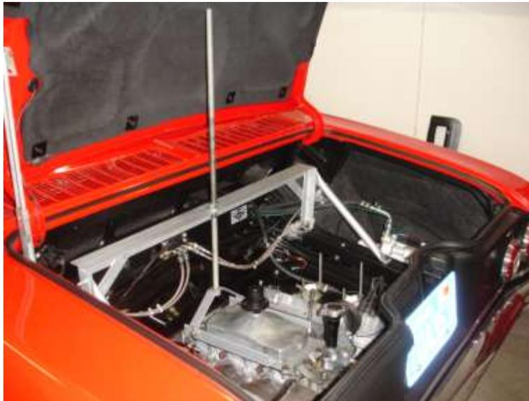
It's called an engine trapeze and it's used to remove or install Corvair power trains. A friend of mine put one together about 35 years ago. He gave me the measurements and I built the one in the picture.
