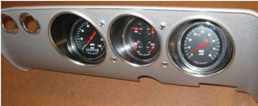
Pretty nice looking don't you think? Notice the two small upper lights between the gauges. Those are LEDs that replace the Temp/Press and Gen/Fan lights in the stock gauges. The gauges from Classic Instruments are mounted to a piece of aluminum which is attached to the back of the LM dash. Here's a picture.
