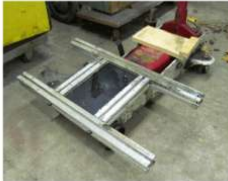
Left: The finished cradle on the floor jack. Below: The cradle in place ready to support the Corvair drive train.
