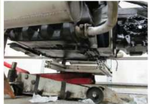
Left: A bottom view of the cradle showing the round steel bar welded in the center of the plate. The diameter of the bar needs to be able to fit into the hole in the floor jack.
