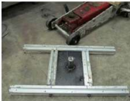
Left: A bottom view of the cradle showing the round steel bar welded in the center of the plate. The diameter of the bar needs to be able to fit into the hole in the floor jack.
