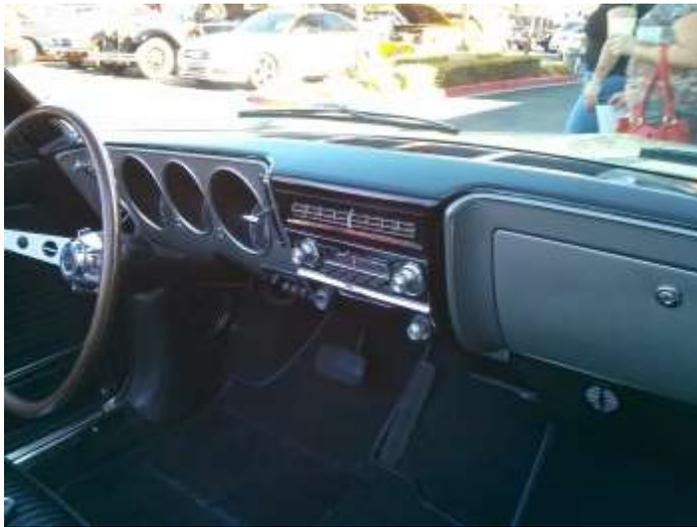
In dash air conditioning, telescoping steering wheel, AM/FM stereo were a few of the upgrades made available in the 1965 Chevy Corvair Monza.
